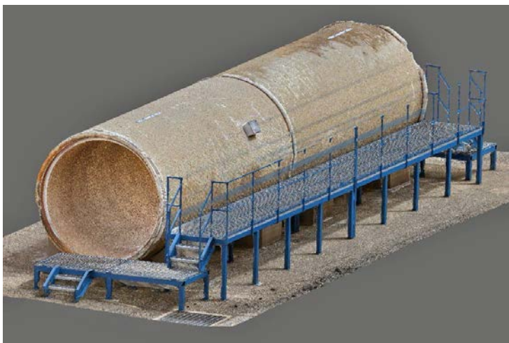
PCCP educational demonstration virtual model created by photogrammetry.
