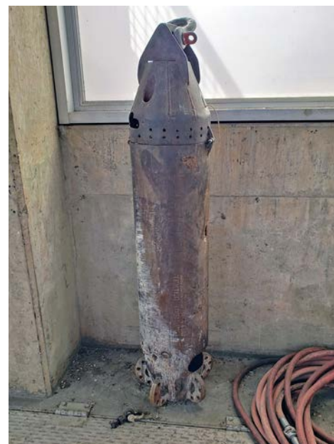
Hoover Dam's sealant deployment device.
