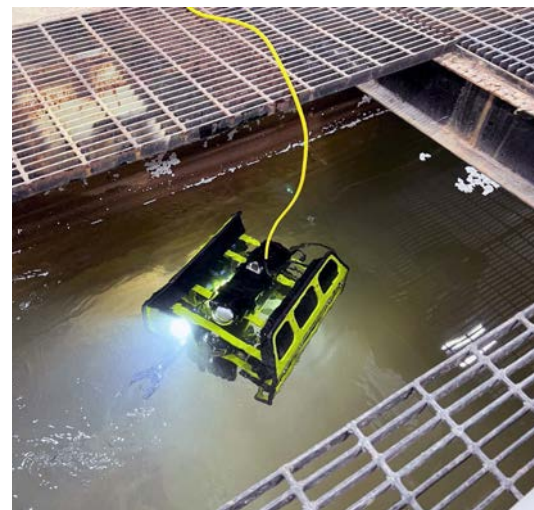
Operation of the UNRD Prosecutor Gen 2 ROV at the Hydraulics Lab sump pool.
