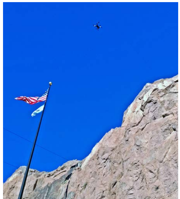
Uncrewed aerial system (UAS) collecting data on Hoover Dam rockfaces to identify rock fall hazards has a 12.2 benefit-cost ratio.
